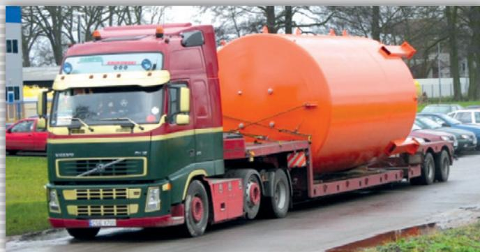
Special tank 51 m<sup>3</sup> diameter 3200 mm
