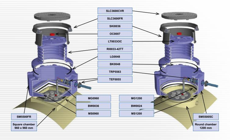
The SM5500 sump base is available with plain bottom for cut-out on site to match the provided tank frame.
