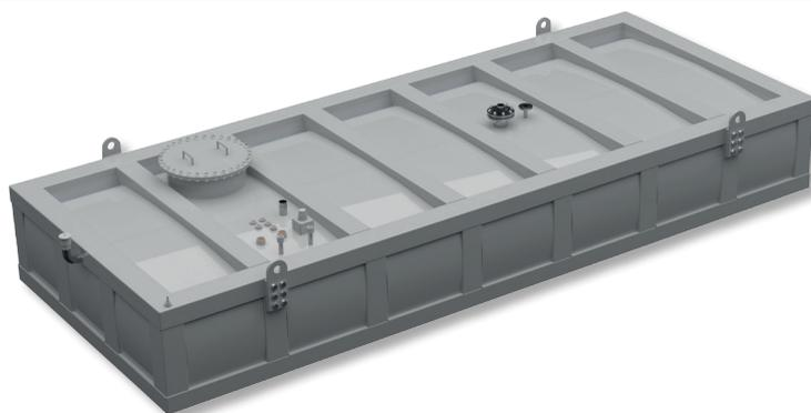
Belly tanks are used as backup fuel storage tanks to supply emergency power generators for data centres. They can be designed to carry the weight of a generator or a container and can also be placed next to the unit. CGH Group also supplies cylindrical tanks.
